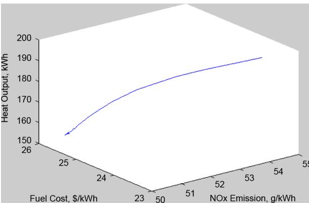
Fig. 5. 3-D plot of optimal front showing the relations among fuel cost,  $\text{NO}_x$  emission, and heat demand at 169-kW electric demand tracking with PSO.
