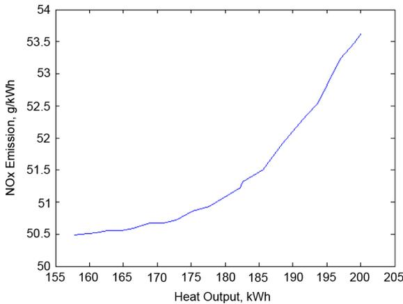
Fig. 6. Heat output versus  $\text{NO}_x$  emission at 169-kW electric demand.
