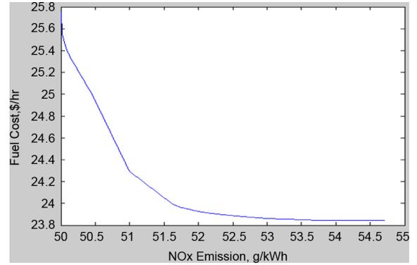
Fig. 2. Pareto optimal front for fuel cost and NO<sub>x</sub> emission at 169-kW electric demand with DE.
