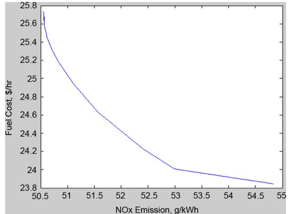
Fig. 3. Pareto optimal front for fuel cost and NO<sub>x</sub> emission at 169-kW electric demand with PSO.
