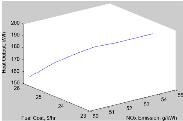
Fig. 4. 3-D plot of optimal front showing the relations among fuel cost,  $\text{NO}_x$  emission, and heat demand at 169-kW electric demand tracking with DE.
